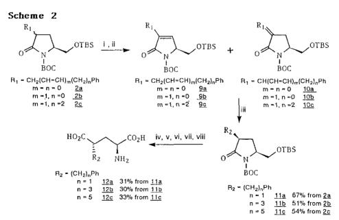
(i) LDA, -78 $^{\circ}$ C, PhSeCI (ii) 30% H<sub>2</sub> O<sub>2</sub> , 0 $^{\circ}$ C (iii) H<sub>2</sub> , 10% Pd/C (iv) 2.5 eq. LiOH, THF, H<sub>2</sub>O 0 $^{\circ}$ C to room temp. (v) PTSA, MeOH, room temp. (vi) 1N NaOH, THF, H<sub>2</sub>O, 0 $^{\circ}$ C (viii) Jones Oxidation, 0 $^{\circ}$ C (viii) TFA, CH<sub>2</sub>Cl<sub>2</sub> 0 $^{\circ}$ C
