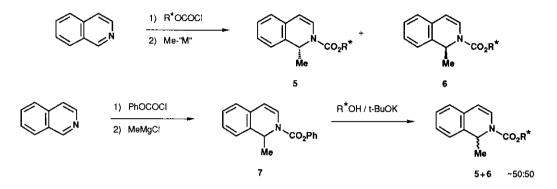
Of the classical methyl Grignard reagents, methylmagnesium iodide gave the best result effecting an 80% yield and 64% de (entry f). Two attempts at raising the asymmetric induction by increasing the bulk of the
