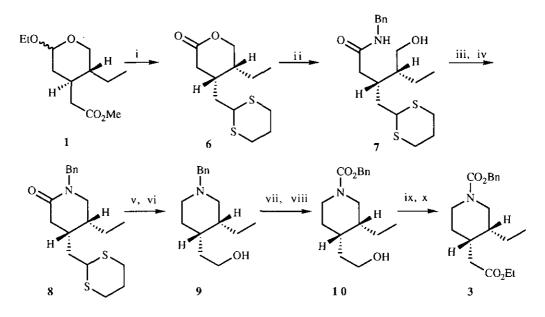
Reagents and conditions: i, 1, 3-propanedithiol, BF<sub>3</sub>·Et<sub>2</sub>O; ii, benzylamine, heat; iii, MsCl, Et<sub>3</sub>N; iv, KH, 18-crown-6; v, MeI, NaHCO<sub>3</sub>; vi, LiAlH<sub>4</sub>; vii, 10% Pd-C, HCO<sub>2</sub>NH<sub>4</sub>, viii, ClCO<sub>2</sub>Bn, NaHCO<sub>3</sub>; ix, CrO<sub>3</sub>, H<sub>2</sub>SO<sub>4</sub>, acetone; x, conc. H<sub>2</sub>SO<sub>4</sub>, EtOH.
