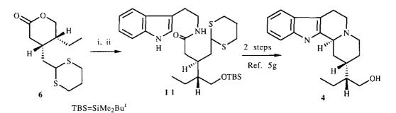
Reagents and conditions: i, tryptamine, heat; ii, TBSCl, Et<sub>3</sub>N, DMAP.
