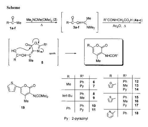
To prepare the compound (3a), acetal (2) was refluxed with a four-fold molar excess of acetone (1a), then the volatile components were removed under reduced pressure and the crude compound (3a) was used for further transformation. This modification is required due to high volatility of acetone, which therefore must be present in the reaction mixture in a large excess. Compounds (3a-f) are known from the literature and have been prepared by a variety of methods.<sup>7</sup>
