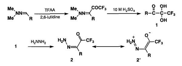
acetylation at azomethine carbon atom. Thus obtained monohydrazones (2) are characterized by strong push-pull type electronic structure indicated above and expected as a good building block for construction of several fluorine-containing heterocycles.
