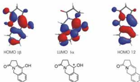
Figure 2. HOMO of 12 (R=H) and enol (1β) (R=H) and LUMO of cation (1α) (R=H) by DFT B3LYP/6-311+G. 28
