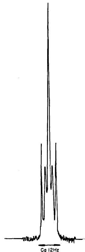
Figure 1.—Methyl resonance pattern observed in the nmr spectra of {Rh[P(OCH 3 ) 2 C 6 H 5 ] 4 }PF 6 and {Rh[POCH 3 (C 6 H 5 ) 2 ] 4 }PF 6 .
