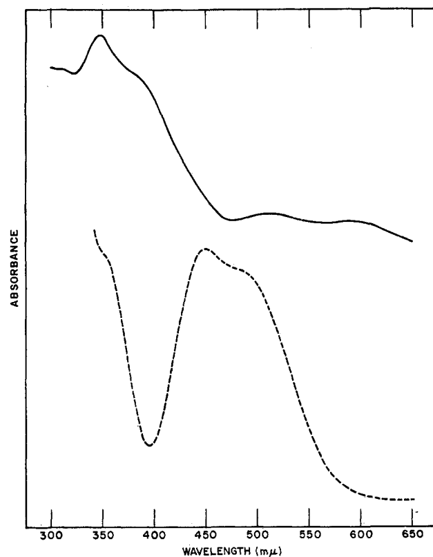
Figure 1.—Visible spectra of [Fe(Et 2 dtc) 3 ] (—) and [Fe( i -Pr 2 dtc) 2 ]BF 3 (---) in methylene chloride solution.
