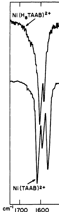
Figure 1.—Infrared spectral bands in the double-bond region for \text{Ni}(\text{TAAB})^{2+} and \text{Ni}(\text{H}_8\text{TAAB})^{2+} .
