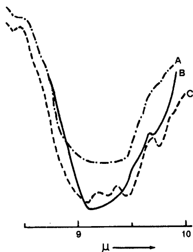
Figure 2.—Infrared spectra of [\text{Cu}(\text{DBen})_2](\text{ClO}_4)_2 \cdot \text{H}_2\text{O} (A), [\text{Cu}(\text{DBen})_2\text{Br}]\text{ClO}_4 (B), and [\text{Cu}_2(\text{DBen})_4(\text{SCN})(\text{ClO}_4)_2]\text{ClO}_4 (C).
