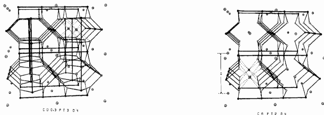
Figure 2. Crystal structures of \text{Cd}_{0.3}\text{Pt}_3\text{O}_4 (general bronze structure) and \text{CaPt}_2\text{O}_4 (from ref 1b). The oxygen and platinum atoms are drawn as open and solid circles, respectively. The coordination of oxygen around the counterions is shown in the upper right-hand corner (for \text{Cd}_{0.3}\text{Pt}_3\text{O}_4 ) and in the lower left-hand corner (for \text{CaPt}_2\text{O}_4 ).
