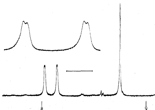
Figure 1. ^1\text{H} NMR spectrum, in the upfield region, of the complex \text{BupyCo}(\text{DH})_2\text{P}(\text{O})(\text{OCH}_3)(\text{C}_6\text{H}_5) [ \text{CH}_2\text{Cl}_2 , 5% TMS, HA100 (100 MHz)]. The bar is 25 Hz long in the lower trace (downfield multiple) (\text{DH})_2 methyl resonance, upfield singlet butyl resonance and is 5 Hz long for the inset, which is an expansion of the (\text{DH})_2 resonance. The numbers are \tau values; TMS reference.
