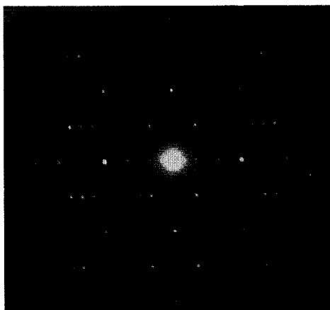
Figure 1. Electron diffraction pattern of 9H-BaIrO 3 , with the beam along \langle 10\bar{1}0 \rangle .
