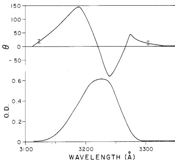
**Figure 1.** Low-resolution absorption and MCD spectra of the  ${}^1A_{1g} \rightarrow {}^1E_u(\pi) + {}^1A_{2u}$  transitions in  $\text{AuCl}_4^-:\text{Cs}_2\text{NaYCl}_6$  at  $\sim 10$  K.  $\theta$  is in millidegrees. The MCD spectrum was recorded at  $H = 55$  kG. All spectra have been digitized by hand. The noise level is equivalent to the pen width in absorption and is shown as error bars for the MCD.
