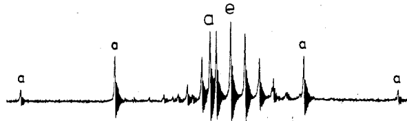
Figure 4. The ^{11}\text{B} NMR spectrum of a mixture of \text{NaBH}_4 (a) and \text{NaBD}_4 (e) in 1.0 M NaOH/ \text{H}_2\text{O} . H-D exchange is absent. The center of the \text{BD}_4^- resonance occurs upfield of the center of the \text{BH}_4^- resonance. Features due to \text{NaBHD}_3 impurity in the \text{NaBD}_4 sample are weakly visible.
