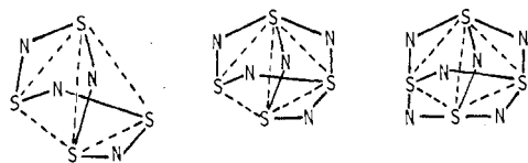
Figure 1. Structures of S 4 N 4 , S 4 N 5 - , and S 4 N 6 2- .
