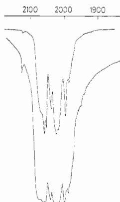
Figure 9. \nu(\text{CO}) infrared spectra of polycrystalline \text{Ru}_2\text{Os}(\text{CO})_{12} (KBr disk, two concentrations).
