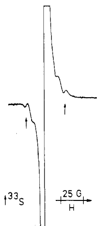
Figure 2. X-Band single-crystal EPR spectrum of (n\text{-Bu}_4\text{N})[\text{}^{61}\text{Ni}/\text{Au}(\text{mnt})_2] . The magnetic field is located perpendicular to the b axis (nearly coincident with the direction of g_z ). T = 295 K.
