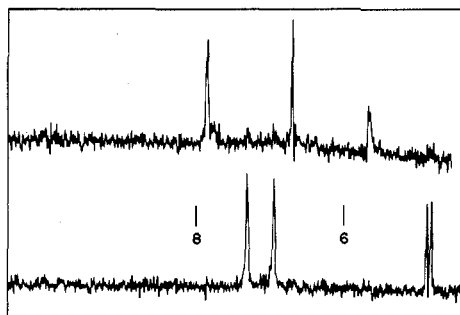
Figure 2. Proton NMR spectrum of \text{enPd}^{2+}\text{IMP}^{3-} (top) compared to that of free \text{IMP}^{2-} at pH 8 (bottom). The vertical lines designate chemical shifts 8.00 and 6.00 ppm downfield from tert -butyl alcohol as an internal reference.
