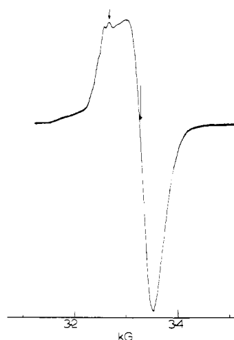
Figure 2. X-Band ESR spectrum of a CH 2 Cl 2 glass (-180 °C) containing electrochemically generated [Mo 2 Cl 4 (P- n -Pr 3 ) 4 ] + .
