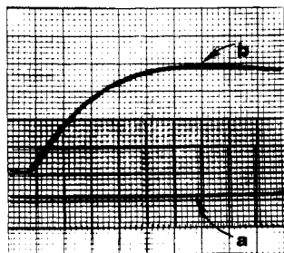
Figure 1. Stopped-flow control experiments. Trace a is a (reversed) oscillograph of an experiment in which a buffered iodine solution containing iodate is mixed with buffer. No reaction is detected. Experimental data: [I_2] = 2.74 \times 10^{-4} M, [IO_3^-] = 9.3 \times 10^{-5} M, pH 3.0, acetic acid-acetate buffer. Trace b is with the same solutions mixed as in a but with no iodate added to the iodine solution. Note the delay time before the trace begins to rise. The vertical axis is proportional to increasing transmittance at 460 nm. The horizontal axis is increasing time, 0.5 s/major division.
