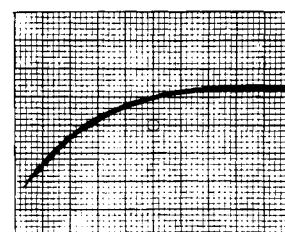
Figure 3. Oscillograph of stopped-flow experiment assigned to oxidation of iodine by chlorite. Experimental data: [I_2] = 3.42 \times 10^{-4} M, [ClO_2^-] = 1.5 \times 10^{-2} M, [IO_3^-] \approx 10^{-4} M, pH 3.31. Oscillograph: vertical axis 50 mV/major division, 0–100% transmittance = 500 mV; horizontal axis 100 ms/major division.
