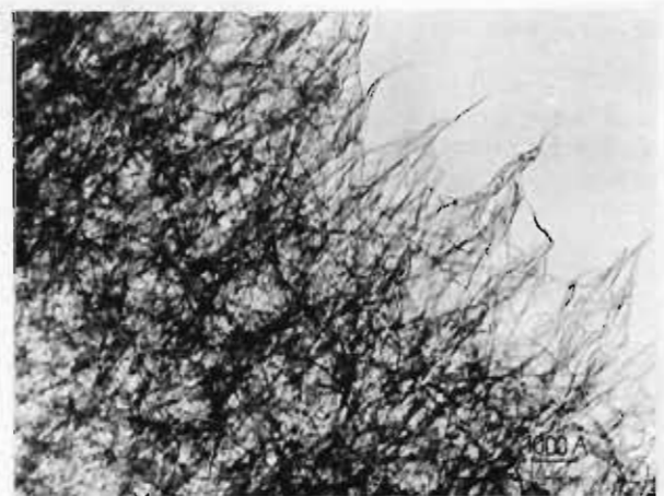
Figure 8. Electron micrograph of polyvanadic acid gel showing the polymeric texture of the condensed species.
