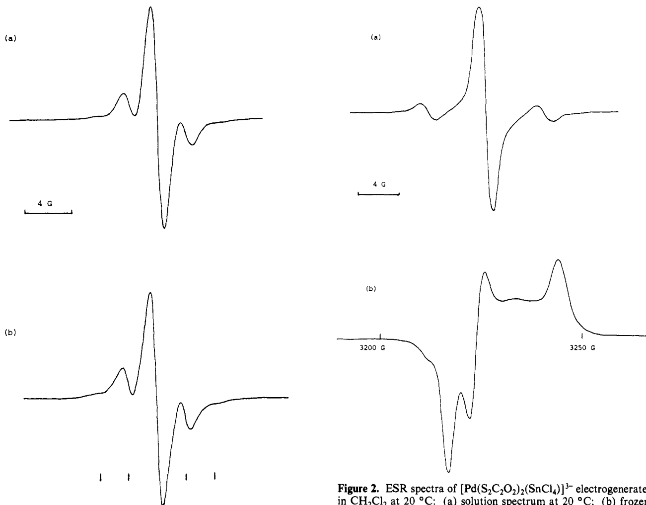
Figure 1. ESR spectra of [Ni(S_2C_2O_2)_2(SnCl_4)_2]^{3-} electrogenerated in CH_2Cl_2 at 17 °C: (a) experimental; (b) simulated (parameters given in Table IIA). The stick spectrum shows the position of satellites due to 7% of two magnetic tin isomers and 13.7% of one magnetic tin isomer.
