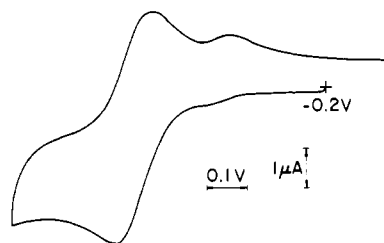
Figure 3. Cyclic voltammogram of 2.50 mM C_{10}H_9Fe(CH_2)_2NMe_2BuBr in 0.8:1 melt (40 °C, Al (2:1) reference, 0.0573 cm^2 vitreous C electrode, scan rate 50 mV s^{-1} ).
