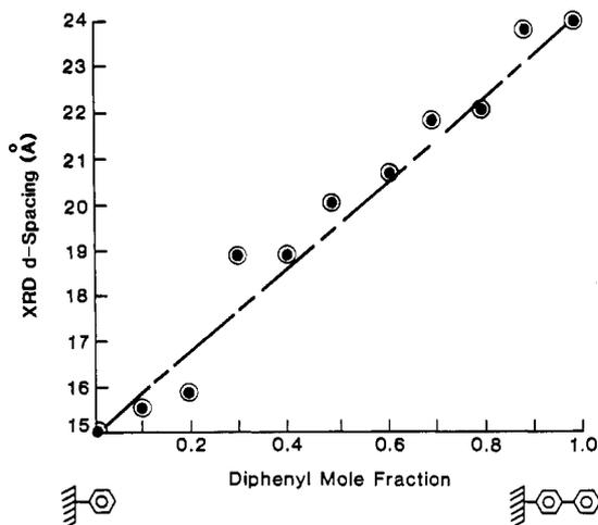
**Figure 4.** Dependence of the layer-layer spacing on compositional variation.
