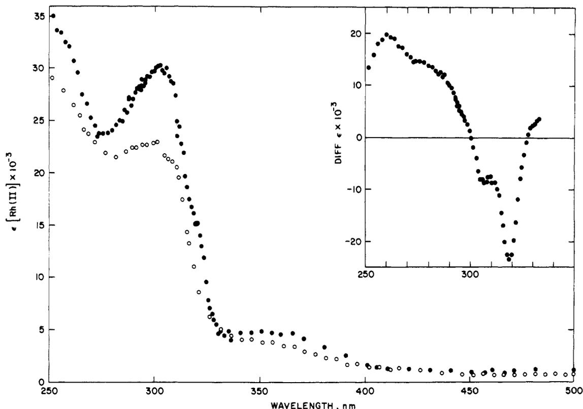
**Figure 1.** Spectra of Rh(II) complexes prepared by reduction of  $(1-2) \times 10^{-5}$  M Rh(III) complexes in 0.013 M 2-propanol at pH 8.8: (●)  $\text{Rh}(\text{bpy})_3^{2+}$ ; (○)  $\text{Rh}^{\text{II}}(\text{bpy})_2(\text{aq})$ . The units of the extinction coefficients are  $\text{M}^{-1} \text{cm}^{-1}$ . The spectra were obtained by adding that of the parent Rh(III) complex to the observed difference spectrum (shown for  $\text{Rh}(\text{bpy})_3^{2+}$  in the insert).
