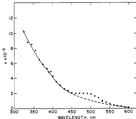
**Figure 5.** Spectrum of the  $\text{Rh}^{\text{II}}(\text{bpy})_2$  dimer ( $\epsilon$  per rhodium) at pH 12 obtained by adding the spectrum of parent  $\text{Rh}(\text{bpy})_2(\text{OH})_2^+$  to the observed difference spectrum.
