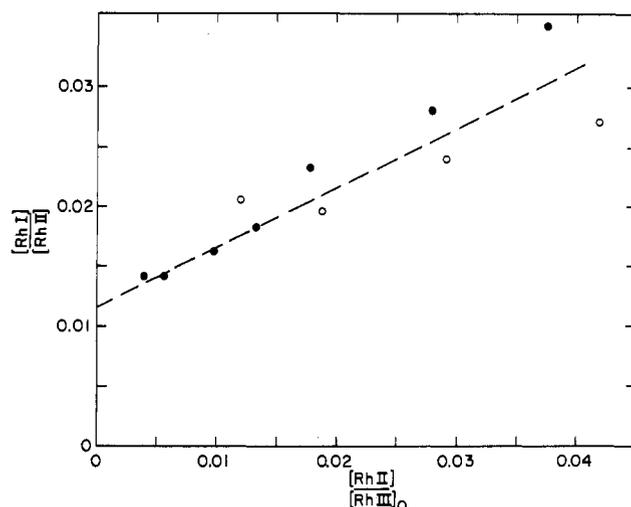
**Figure 3.** Dependence of the yield of  $\text{Rh}(\text{I})$ , produced by radical reduction of  $\text{Rh}(\text{bpy})_3^{2+}$ , on  $\text{Rh}(\text{bpy})_3^{2+}$  and  $\text{Rh}(\text{bpy})_3^{3+}$  concentrations: (●)  $10^{-3} \text{ M Rh}(\text{bpy})_3^{3+}$ ; (○)  $3 \times 10^{-4} \text{ M Rh}(\text{bpy})_3^{3+}$ .
