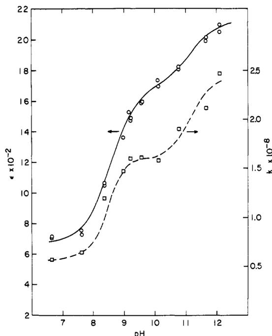
**Figure 2.** Dependence of the  $\text{Rh}^{\text{II}}(\text{bpy})_2(\text{aq})$  extinction coefficient at 390 nm on pH (circles) and the dependence of the dimerization rate constant,  $k_9$  ( $\text{M}^{-1} \text{s}^{-1}$ ), on pH (squares).
