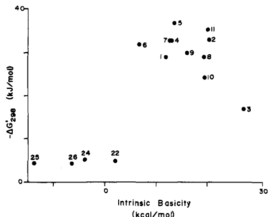
Figure 2. Correlation of the observed free energy of adsorption with literature values for the intrinsic basicity (gas phase \delta_R\Delta G'_{i(g)} values relative to ammonia; see ref 12).
