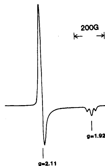
Figure 5. EPR spectrum of [Rh 2 (ac)(acam) 3 ] + in acetonitrile (0.1 M TBAP) at 77 K.
