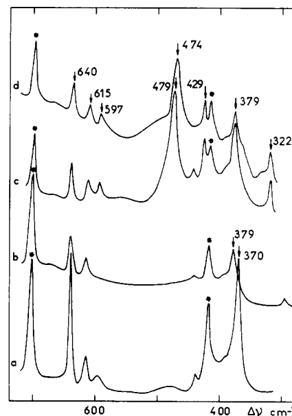
Figure 2. Low-frequency RR spectra of iron(II) picket fence porphyrins in \text{C}_6\text{H}_5\text{Cl} solutions (solvent bands indicated by S), at -30^\circ\text{C} : (a) \text{Fe}(\text{TpivPP})(\text{C}_6\text{HF}_4\text{S}^-)\text{Na}^+18\text{C}_6 , \lambda_0 = 454.5\text{ nm} ; (b) \text{Fe}(\text{TpivPP})(\text{C}_6\text{HF}_4\text{S}^-)(\text{O}_2)\text{Na}^+18\text{C}_6 , \lambda_0 = 440\text{ nm} ; (c) \text{Fe}(\text{TpivPP})(\text{C}_6\text{HF}_4\text{S}^-)(^{13}\text{CO})\text{Na}^+18\text{C}_6 , \lambda_0 = 454.5\text{ nm} ; (d) \text{Fe}(\text{TpivPP})(\text{C}_6\text{HF}_4\text{S}^-)(^{13}\text{CO})\text{Na}^+18\text{C}_6 , \lambda_0 = 454.5\text{ nm} .
