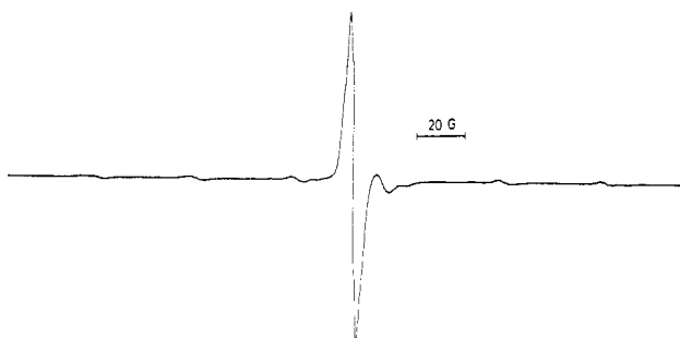
Figure 5. Solution EPR spectrum of sodium naphthalide reduction of [\text{Si}(\text{CH}_3)_2(\text{C}_5\text{H}_4)_2]\text{ZrCl}_2 in THF.
