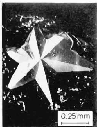
Figure 1. Crystals of In 11 Mo 40 O 62 exhibiting the twinning pattern that is characteristic for the compound. All crystals are threefold twinned.
