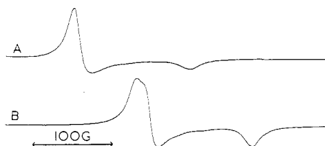
Figure 3. ESR spectral envelopes (300 K) of polycrystalline (C_4H_9)_4N^+Ni(bds)_2^- (A) and (C_4H_9)_4N^+Ni(bdt)_2^- (B). The spectra are shown in the correct magnetic field relationship, i.e., the field increases left to right.
