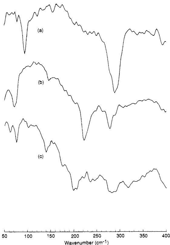
Figure 2. Far-infrared spectra: (a) (PPh 2 - o -tol) 2 CuCl; (b) (PPh 2 - o -tol) 2 CuBr; (c) (PPh 2 - o -tol) 2 CuI.
