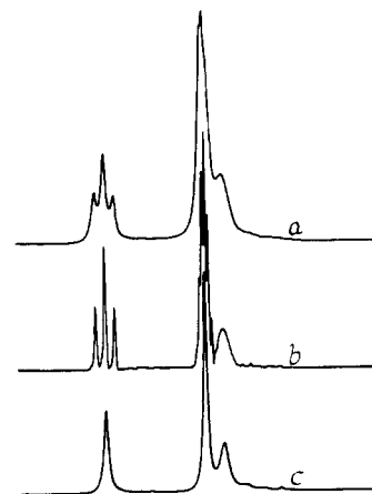
Figure 1. 86.7-MHz 11 B NMR spectra of neat (\mu\text{-Me}_2\text{N})_2\text{B}_4\text{H}_8 : (a) normal; (b) line narrowed; (c) 1 H decoupled.
