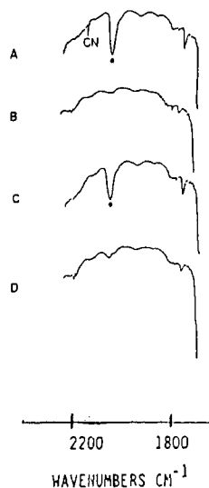
Figure 3. FT-IR spectra of [P]-N(CH 3 ) 2 CuCl: (A) after exposure to 25 psig of CO (solvated complex; the asterisk indicates CO stretch at 2065 cm -1 ); (B) after evacuation; (C) after exposure to 26 psig of CO; (D) after evacuation and exposure to air and then 2k psig of CO.
