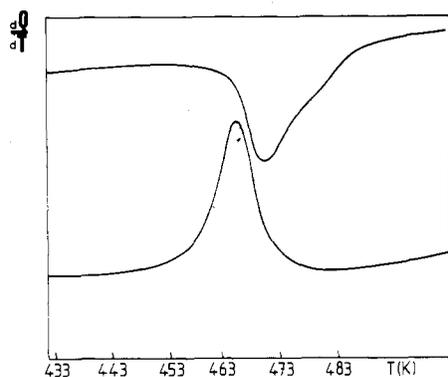
Figure 4. DSC study of the  $\text{Mg}_2\text{CoH}_3$  phase transformation from the tetragonal to the cubic variety.
