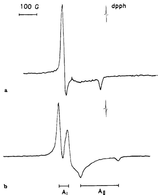
**Figure 4.** Frozen solution ESR spectra at 77 K in aqueous media: (a)  $[\text{Ni}^{\text{III}}(\text{L1})(\text{H}_2\text{O})]^{3+}$ ; (b)  $[\text{Ni}^{\text{III}}(\text{L1})(\text{F})]^{2+}$ .
