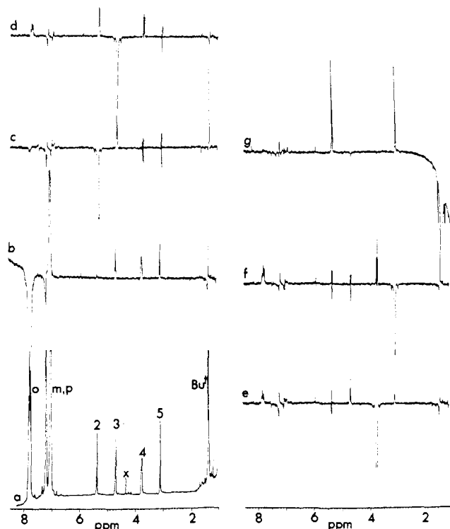
Figure 2. NOe spectra for [(\eta^5\text{-C}_5\text{H}_4\text{Bu}^1)\text{Fe}(\text{CO})(\text{PPh}_3)\text{I}] : (a) nonirradiated, where o, m, and p represent signals corresponding to the ortho, meta, and para protons on the \text{PPh}_3 phenyl rings, 2–5 represent signals for the protons \text{H}_2\text{--H}_5 on the Cp ring, and \text{Bu}^1 represents the signal for the protons on \text{Bu}^1 ; (b) irradiated ortho phenyl ring proton ( \text{H}_o ); (c) irradiated ring proton \text{H}_2 ; (d) irradiated ring proton \text{H}_3 ; (e) irradiated ring proton \text{H}_4 ; (f) irradiated ring proton \text{H}_5 ; (g) irradiated \text{C}_5\text{H}_4\text{Bu}^1 . Absorption marked \times is an impurity peak.
