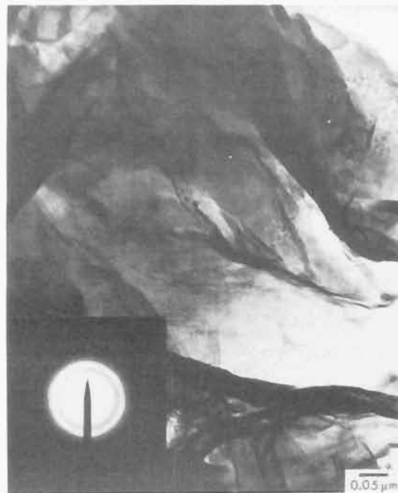
Figure 11. Transmission electron micrograph of the Cu/Zn/Cr = 30/45/25 mol % hydrotalcite-type precursor and the corresponding selected area diffraction pattern.
