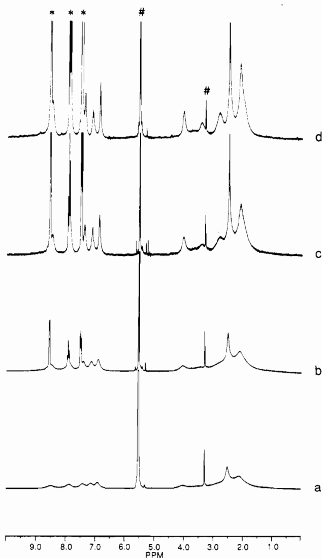
Figure 4. ^1\text{H} NMR spectra of [\text{Ag}(\text{5MeTh-Met-Histam})](\text{OTf}) [ c = 0.11\text{ mol}\cdot\text{L}^{-1} , in CD 3 OD (#) at 233 K with added pyridine (*): (a) pure complex; (b) complex + 0.25 equiv of pyridine; (c) complex + 1.0 equiv of pyridine; (d) complex + 2.0 equiv of pyridine.
