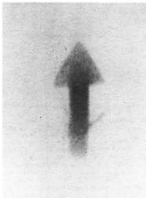
Figure 1. Spatially structured film of poly- \text{Ru}(\text{vbpy})_3^{m+} grown on antimony-tin oxide coated glass via Scheme I. (Structure dimensions are 12 mm by 5 mm.)
