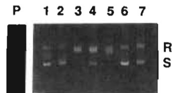
Figure 1. The relaxation of supercoiled plasmid (pAXHP) by topoisomerase I was monitored by agarose gel electrophoresis (S = supercoiled, R = relaxed). 7 Each lane represents activation by a different metal cofactor: (1) \text{Mg}^{2+}(\text{aq}) , (2) [\text{Co}(\text{NH}_3)_6]^{3+} , (3) [\text{Co}(\text{NH}_3)_5(\text{CO}_3)]^+ , (4) [\text{Co}(\text{NH}_3)_5(\text{NO}_2)]^{2+} , (5) [\text{Co}(\text{NH}_3)_5\text{Cl}]^{2+} , (6) [\text{Co}(\text{NH}_3)_5(\text{OH})]^{2+} , (7) [\text{Co}(\text{NH}_3)_5(\text{C}_2\text{O}_4)]^+ . A control lane (P) shows the unreacted plasmid. Reactions with complexes in the absence of enzyme gave no reaction. Each reaction mixture (10 \mu\text{L} ) contained the following: 6 mM \text{M}^{n+} ; 50 mM Tris (pH 8); 50 mM KCl; topoisomerase I (Bethesda Research Laboratory, 2 units); pAXHP (0.5 \mu\text{g} ). After incubation at 0 °C for 30 min, the reaction was terminated with 1 \mu\text{L} of gel-loading buffer (5% bromophenol blue, 5% xylene cyanol EE, 5% orange C, 60% glycerol) and run on a 0.8% agarose gel in 1 \times TAE buffer at 100 V for 45 min. As expected, the data support a processive rather than a distributive mechanism. 2
