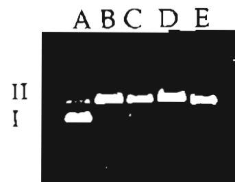
Figure 11. Photograph of a 1% agarose gel showing the results of electrophoresis of 60 \mu\text{M} \phi\text{X174} DNA after electrolysis at 0.8 V in the presence of 40 \mu\text{M} (A) \text{Ru}(\text{bpy})_2(\text{py})\text{OH}_2^{2+} , (B) \text{Ru}(\text{phen})_2(\text{py})\text{OH}_2^{2+} , and (C) \text{Ru}(\text{tpy})(\eta^2\text{-tpt})\text{OH}_2^{2+} and at 0.5 V in the presence of 40 \mu\text{M} (D) \text{Ru}(\text{tpy})(\text{tmen-AO})\text{OH}_2^{3+} .
