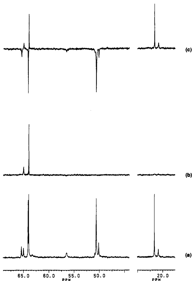
Figure 2. ^{13}\text{C} DEPT NMR spectra of 1 in DMF solution: (a) proton-decoupled ^{13}\text{C} spectrum; (b) 90^\circ pulse for CH; (c) 135^\circ pulse for \text{CH}_3 (positive) and \text{CH}_2 (negative).
