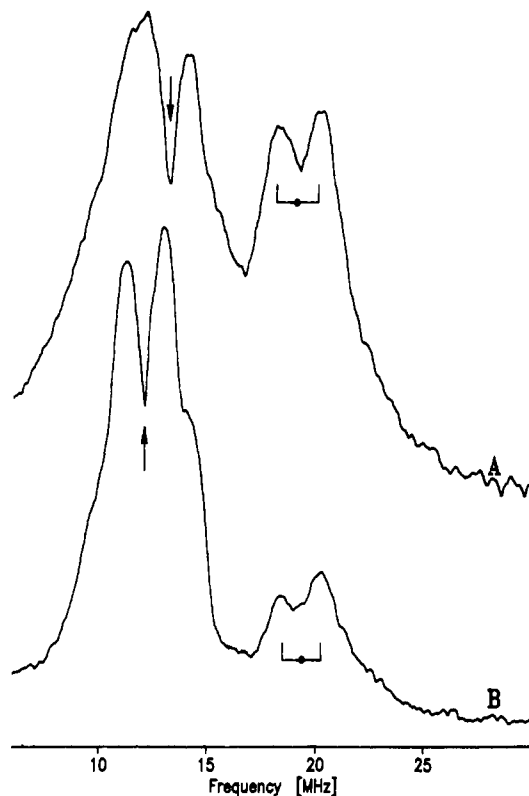
Figure 3. X-band ENDOR spectra of \text{Ag}_{12}\text{Cu}_{112}\text{SOD} at two microwave frequencies, with H_0 set to \sim g_2 . Proton resonances shift with frequency, whereas the ^{14}\text{N} resonances do not. The position of the ^{14}\text{N} resonance is indicated by A^N/2 (•) and 2\nu_N (|—|). Conditions are as follows. A: microwave frequency, 9.525 GHz; H = 0.31 T; T = 2 K; microwave power, 2 \mu\text{W} ; 100-kHz field modulation, 5 G; RF power, 20 W; RF scan rate, 5 MHz/s. B: microwave frequency, 8.7 GHz; H_0 = 0.283 T; other conditions as in (A).
