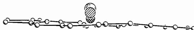
Figure 5. Schematic “overlay” representation of complexes 3 , 37 , and 22 illustrating the variation in distance above the \text{N}_5 plane of the La(III) (dotted circle, 0.91 Å), Gd(III) (lined circle, 0.60 Å) and Lu(III) (cross-hatched circle, 0.27 Å). The Ln(III) ions were oriented by best fitting (i.e., superimposing) the nitrogen donor atoms of the macrocycles by least-squares methods. The conformation of the macrocycle shown is that for lutetium(III) texaphyrin ( 22 ). The cation spheres are scaled to one-fourth of the ionic radii given in Shannon 42 for 10-, 9-, and 8-coordinate \text{La}^{3+} (1.27 Å), \text{Gd}^{3+} (1.11 Å), and \text{Lu}^{3+} (0.98 Å), respectively.
