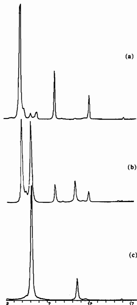
Figure 4. XRD patterns of (a) \alpha -ZrP·2PMA, (b) partially p -H 2 TAPP-exchanged \alpha -ZrP·2PMA, and (c) "fully" p -H 2 TAPP-exchanged \alpha -ZrP·2PMA. Horizontal axis is in degrees 2\theta .
