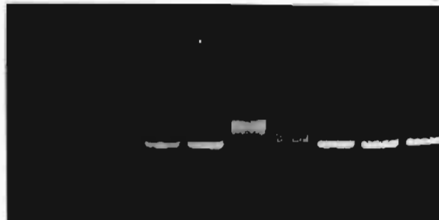
Figure 2. Gel mobility of supercoiled pSP64 (25 \mu g/mL, 40 \mu M bp, all lanes) plasmid DNA in the presence of Ni 2 (14) and Zn 2 (14) at pH 8.0 (EPPS, 10 mM) at 25 °C after incubation for 15 min. Key: lane 1, DNA only (no metal or ligand); lane 2, 500 \mu M Ni 2 (14) 4+ ; lane 3, 50 \mu M Ni 2 (14) 4+ ; lane 4, 5 \mu M Ni 2 (14) 4+ ; lane 5, 0.5 \mu M Ni 2 (14) 4+ ; lane 6, 500 \mu M Zn 2 (14) 4+ ; lane 7, 50 \mu M Zn 2 (14) 4+ ; lane 8, 5 \mu M Zn 2 (14) 4+ ; lane 9, 0.5 \mu M Zn 2 (14) 4+ ; lane 10, DNA only.
