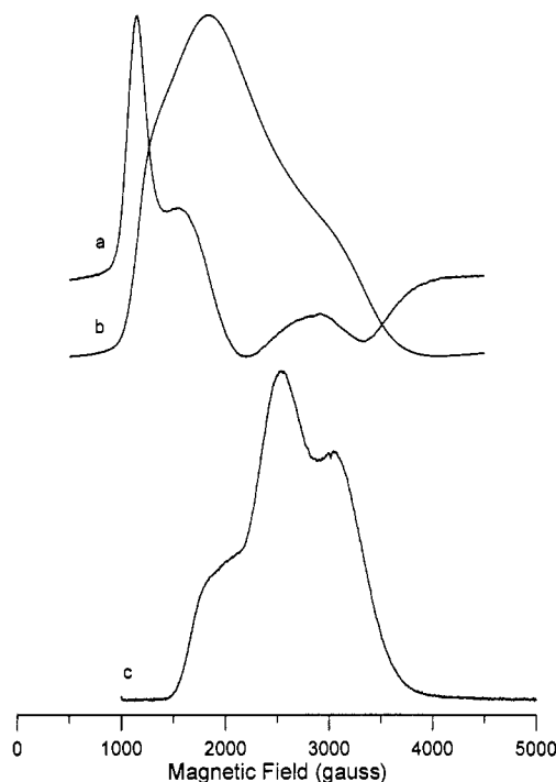
Figure 2. Spectra at X-band (9.2 GHz) of 5.0 mM Co(DTPA) in 1:1 H 2 O:glycerol, pH 5.6. (a) CW spectrum at about 10 K, obtained with 0.1-mW microwave power, 4.0-G modulation amplitude at 100 kHz, scan time of 120 s, average of 2 scans. (b) First integral of spectrum shown in (a). (c) Two-pulse field-swept echo-detected spectrum at about 6.5 K, obtained with 90- \tau -180- \tau -echo sequence with \tau = 150 ns and a 15-ns 90° pulse. The box-car digitizer was sampled 200 times at each magnetic field, and two scans were averaged.
