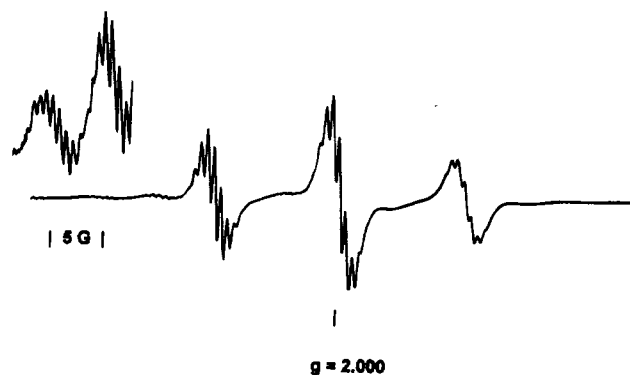
Figure 1. THF solution EPR spectrum of 2a . The insert shows a horizontal and vertical expansion of the Ti hyperfine coupling.
